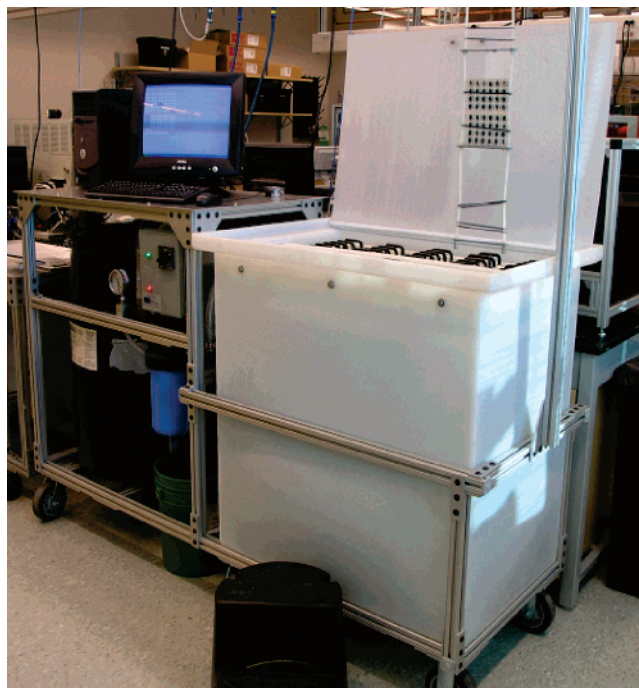
Figure 4. Image of the high-capacity circulating water preconditioning tank. Tank can accommodate up 360 plates simultaneously.
