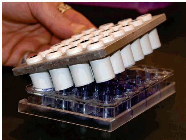
Figure 6. Image of a custom extraction template being applied to a standard 24-well polystyrene plate.
